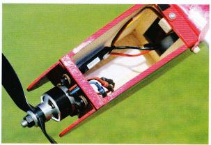
A battery hatch should be easy to create, mine is retained by a small tab. A 3S 850mAh LiPo slips easily inside.
